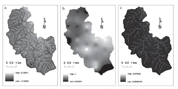
Figure 2. The predicted maps of (a) index of connectivity IC, (b) the maximum theoretical SDR coefficient SDR<sub>max</sub> and (c) SDR variability within the study area. The IC and SDR maps in this figure were selected for spatial variability in 2007. Catchment boundaries are depicted in Figure 1
