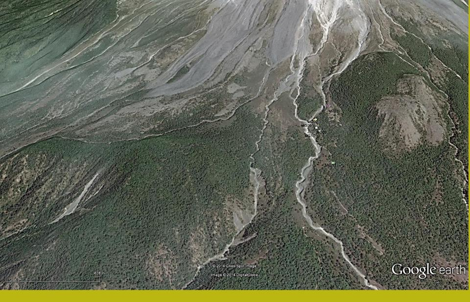
Portion of Colima volcano South flank with several barrancas and main source areas of lahars (above 2500 m a.s.l.); local remobilization, mass movements, and instability of older deposits are in evidence.
