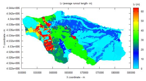
Average run-out length of shallow landslides for each LUS (land unit system) obtained from field survey and multi-temporal aerial photos
